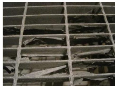
Gratings of Unit 4 of Fukushima Daini (experienced temperature ~150°C)
