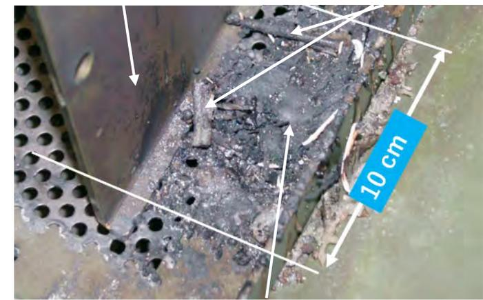
A 10 mm-thick pile of the control blade melt
