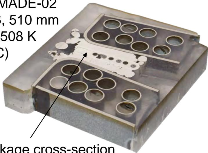
Melt blockage cross-section
