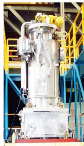
Fig. 7 Mobile Equipment Replacing Cask (hatch type)
