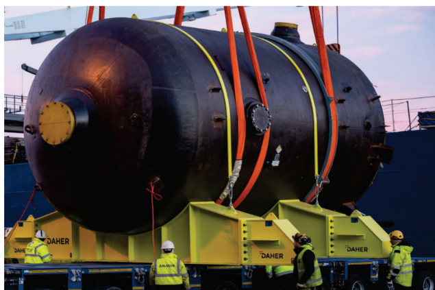
Fig. 4 Arrival of steam generator upper parts for treatment at the on-site harbour (Image courtesy Cyclife)
