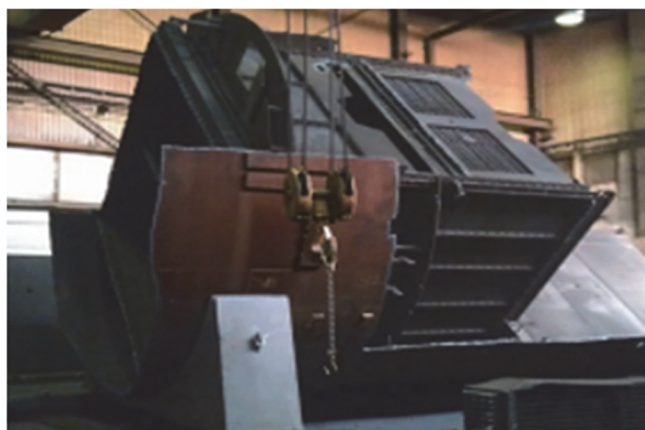
Fig. 10 Partly segmented Magnox boiler
