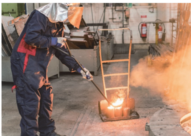
Fig. 7 Casting of the representative samples
