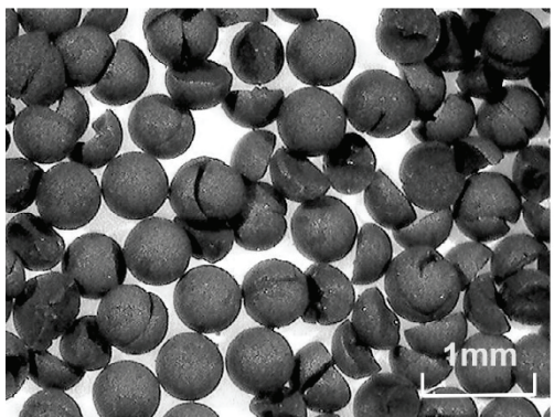
Fig. 9. Photomicrograph of carbon-added dried gel particles with the C/Dy ratio of 1.96 condition
