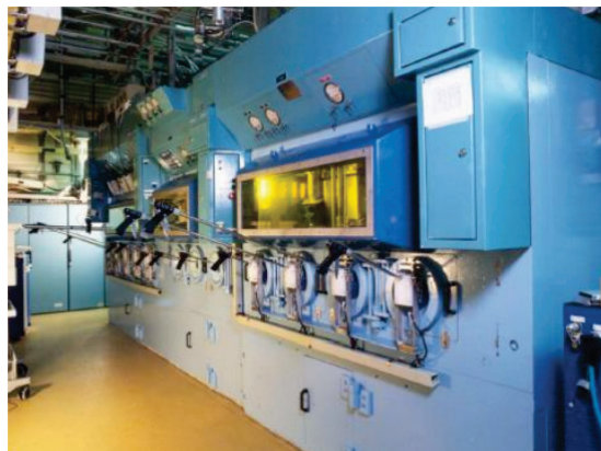
Fig. 2 Shielded hot cells in La Hague reprocessing facility process control laboratory
