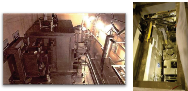
Fig. 9 Left: ANI station in La Hague compaction facility Right: Newly installed ANI station in the Orano La Hague Waste retrieval HAO Cell
