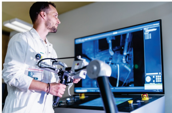
Fig. 5 Computer assisted manipulator used to operate La Hague vitrification facility
