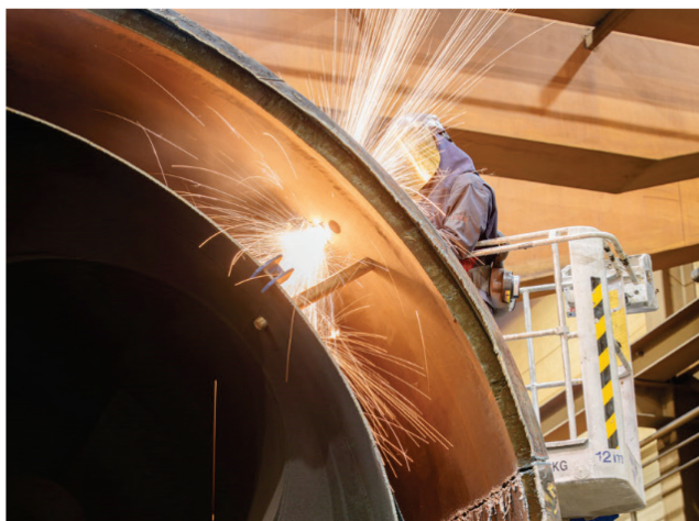
Fig. 5 Segmentation of steam generator upper part (Image courtesy Cyclife)
