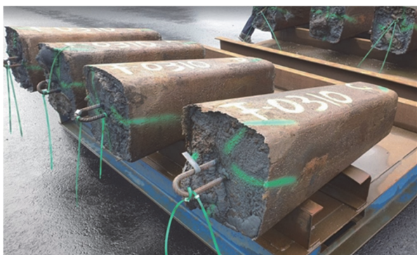
Fig. 9 Ingots ready for release to the conventional metal industry
