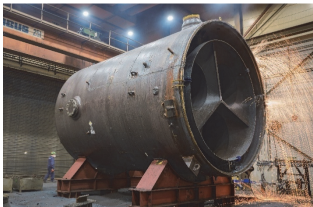
Fig. 11 PWR steam generator upper part in the Cyclife treatment facility
