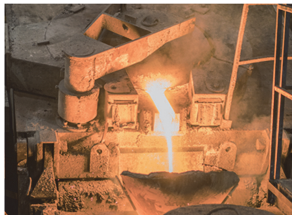
Fig. 8 Casting of ingots
