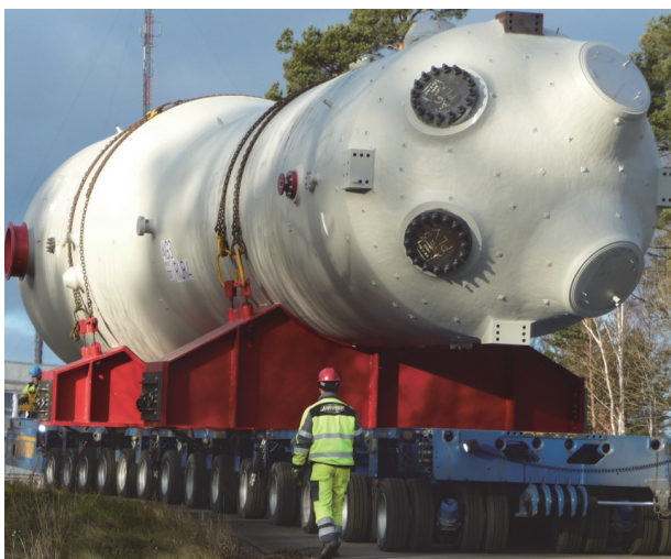
Fig. 3 Arrival of a PWR steam generator to the Cyclife site for treatment
