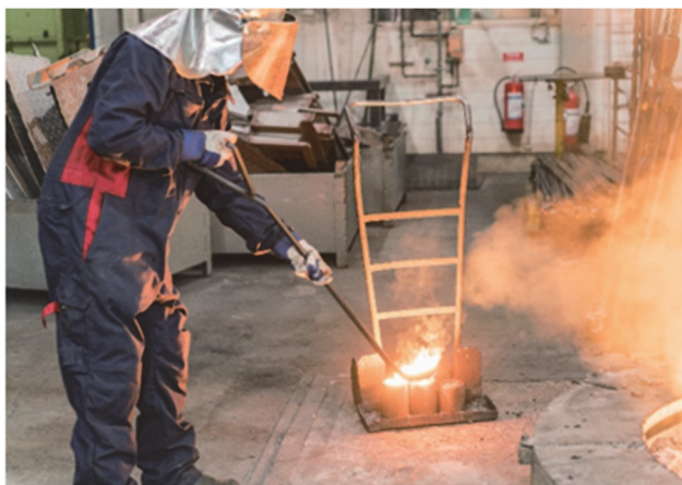
Fig. 7 Casting of the representative samples
