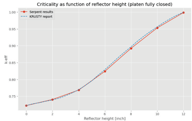
Fig. 8 Criticality as a function of reflector height, assuming a fully inserted platen and no shim reflector.
