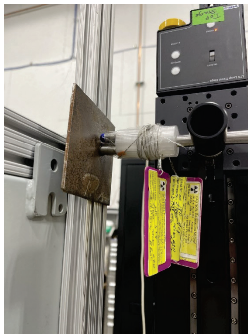
Fig. 3 Detector count rate measurement setup using five neutron sources.
