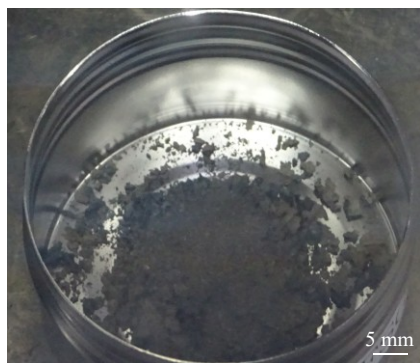
Fig. 1 Appearance of the MA-bearing MOX fuel powder prepared by mixing the MA nitrate solution with the dissolver solution of MOX fuel pellets
