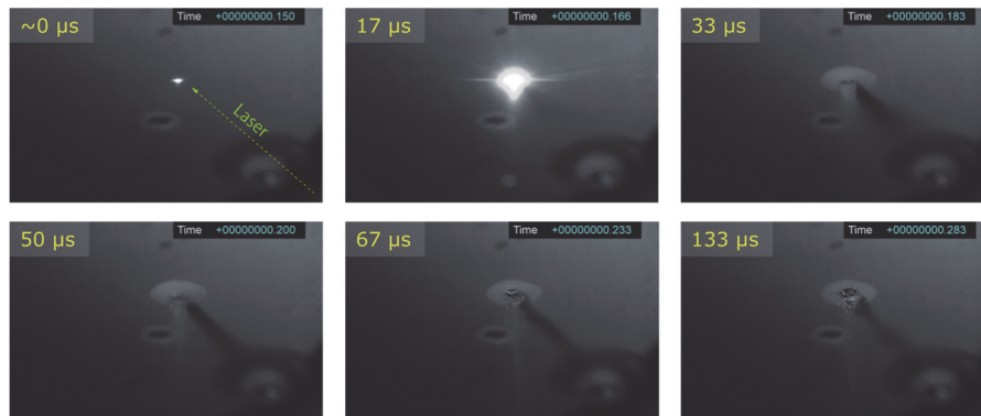
Figure 6. In-situ observation of CO_2 layer during laser ablation using a high-speed camera.
