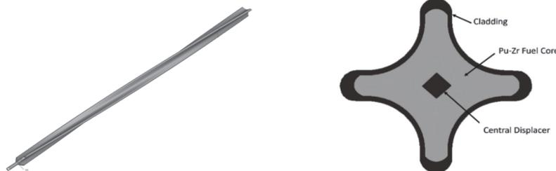
Figure 5. Diagram of Lightbridge's metallic helical cruciform geometry. (left) Segment of the rod showing the helical twist; (right) cross-section of the U-Zr fuel core, central displacer and cladding. This diagram is not to scale.
