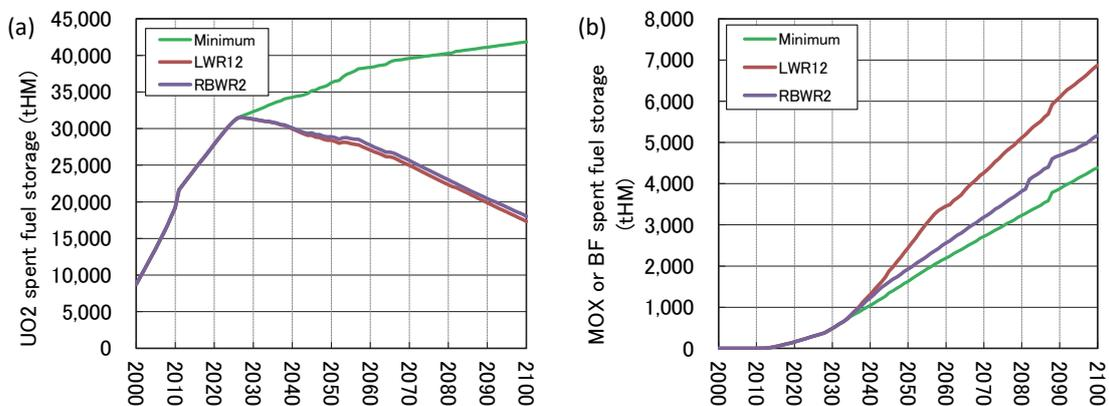
Figure 4. (a) UO<sub>2</sub> SF in storage, (b) MOX or BF SF in storage.
