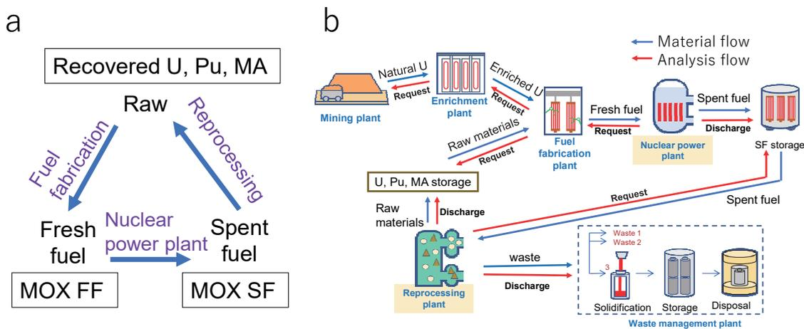
Figure 1. (a) Change of material tags through the plants. (example: mixed oxide (MOX) fuel), (b) Material and analysis flow of NMB4.0.
