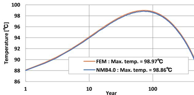
Figure 3. Comparison of the temperature evolution of buffer material for NMB4.0 and FEM.
