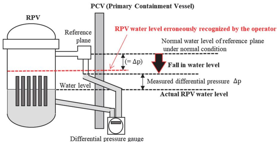
Figure 1. Schematic diagram of differential pressure gauge.
