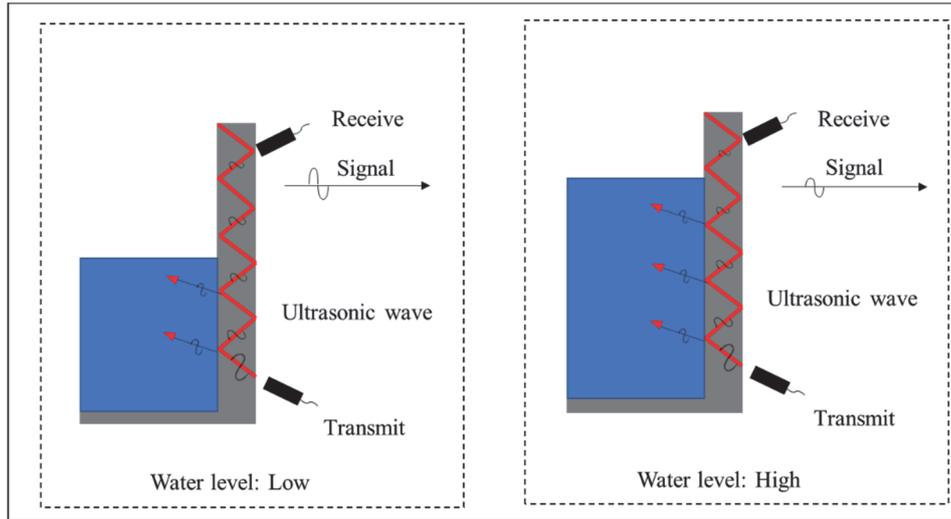
Figure 2. Schematic diagram of ultrasonic clamp-on water level gauge.
