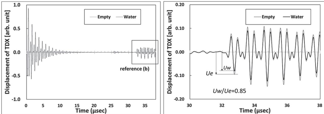
Figure 3. Waveforms of received signals when ultrasonic waves are injected perpendicularly to the vessel.
