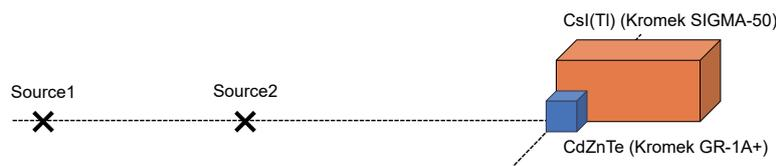
Figure 2. Experimental set-up for performance evaluation of  $^{137}\text{Cs}$  detections and radioisotope identifications. Measurements were made for single or paired sources placed at the same dose rate ( $0.44 \mu\text{Sv/h} \pm 2\sigma$ ) from individual sources.
