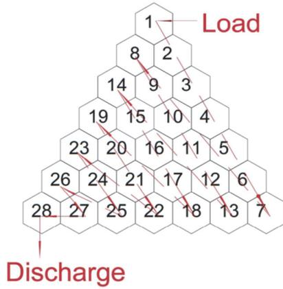
Figure 2. Shuffling pattern in a symmetrical region (one-sixth) of the core.
