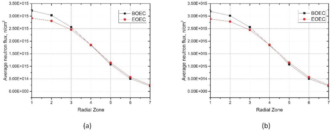
Figure 5. Average neutron flux (a) LBE, (b) lead.
