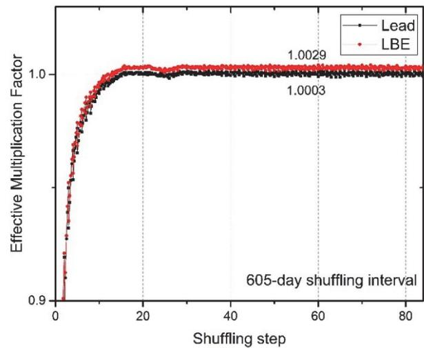
Figure 3. Effective Multiplication Factor during the core shuffling step of LBE/lead.
