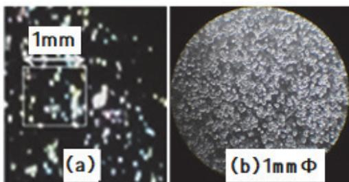
Figure 6. (a) Pit density  $27(\pm 20\%)/\text{mm}^2$  of inner organ of sardine in a small white square shown in Figure 1 (B), and (b) the density  $1637/\text{mm}^2$  of the liver C in Figure 3 (d) of golden threadfin bream.
