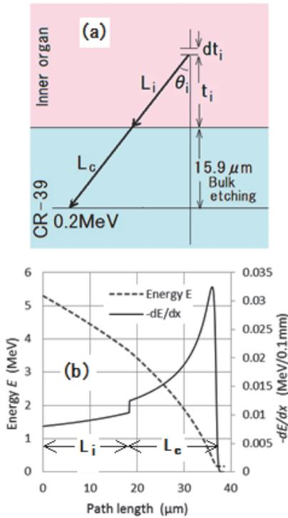
Figure 4. (a) Explanatory picture to calculate detection efficiency of alpha particles emitted in inner organ. The thickness 15.9 μm was a deleted thickness, called bulk etching, of CR-39 by chemical etching. (b) Energy loss (-dE/dx) and energy E calculated by Bethe formula.
