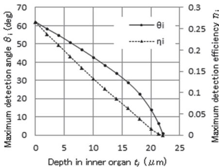
Figure 5. Maximum detection angle  $\theta_i$  and maximum detection efficiency  $\eta_i$  for  $\alpha$ -particle emitted at depth  $t_i$  in inner organ.
