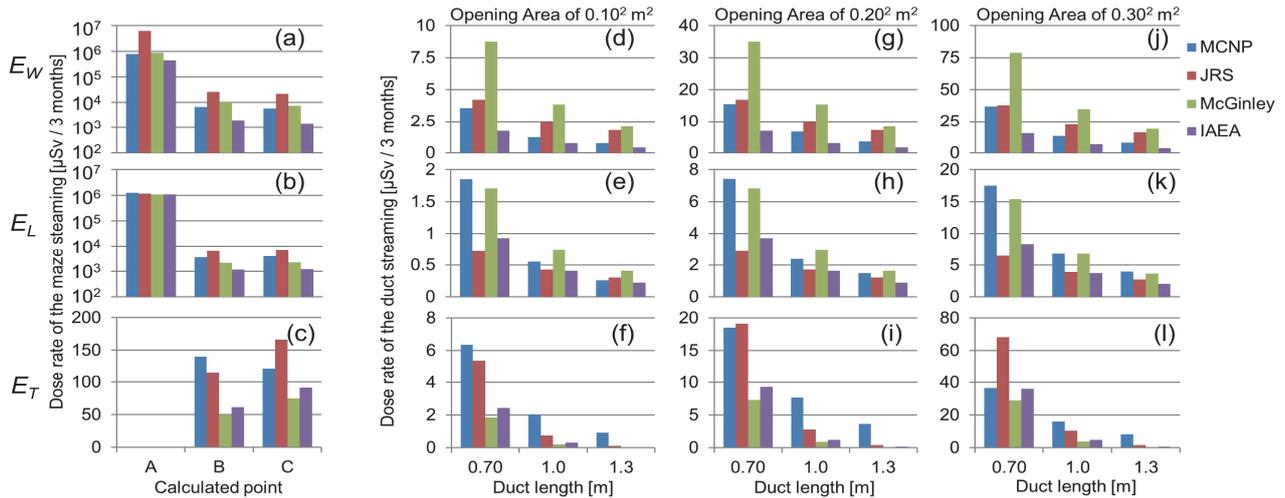
Figure 5. Results of maze streaming (a)-(c) and duct streaming (d)-(l) of X-ray. Streaming paths of (a), (d), (g), and (j) are  $E_W$ , (b), (e), (h), and (k) are  $E_L$  and (c), (f), (i), and (l) are  $E_T$ .
