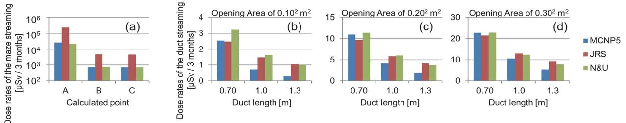
Figure 4. Results of (a) maze streaming and (b)-(d) duct streaming of neutrons. N&U stands for Nakamura & Uwamino’s formula.
