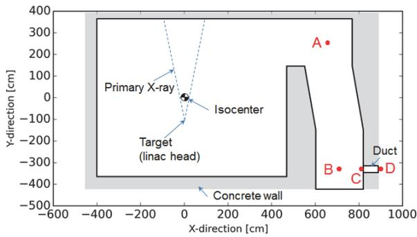
Figure 1. Study room layout and calculation points A, B, C, and D.
