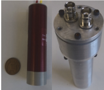
Figure 3. The \text{CeBr}_3 inorganic detector without and with aluminum casing.
