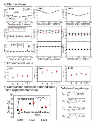
Figure 4. Comparison of doses between the planning system and rectum dosimeter. Figures of a), b), and c) show planned dose, experimental value, and comparison of these data, respectively.
