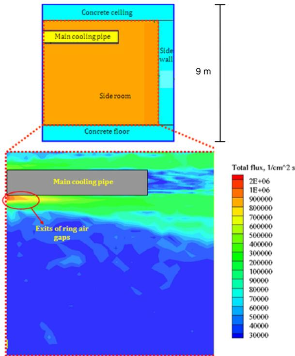
Figure 5. Neutron total flux distribution in a vertical plane parallel to the cooling pipe (reference side room).
