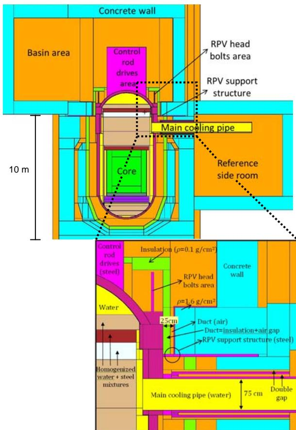
Figure 2. MCNP KKG model (zoom: cooling pipe section).
