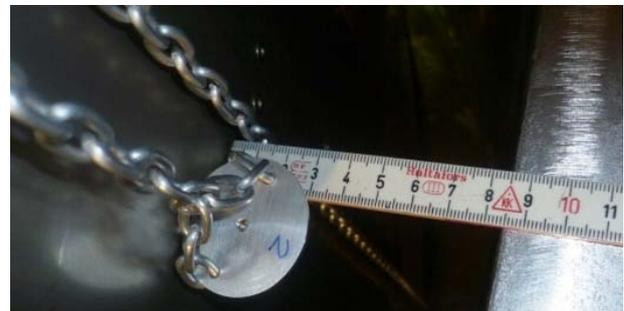
Figure 6. Typical KKG foil sample (at RPV ring gap).
