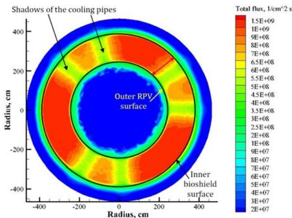
Figure 4. Neutron total flux distribution in a horizontal plane directly above the six cooling pipes.
