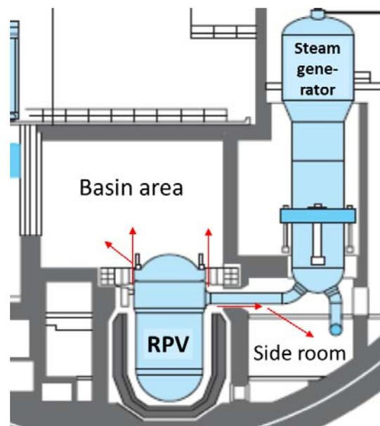
Figure 1. Example of ex-RPV neutron streaming pathways.
