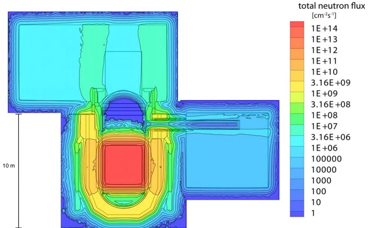
Figure 3. Neutron flux distribution for the extended KKG MCNP model (for a typical middle of cycle situation).
