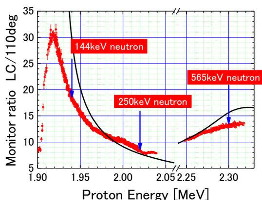
Figure 9. Relationship between proton energy and count ratio of the LC and the 110deg-monitor for  ${}^7\text{Li}(p,n){}^7\text{Be}$  reaction.
