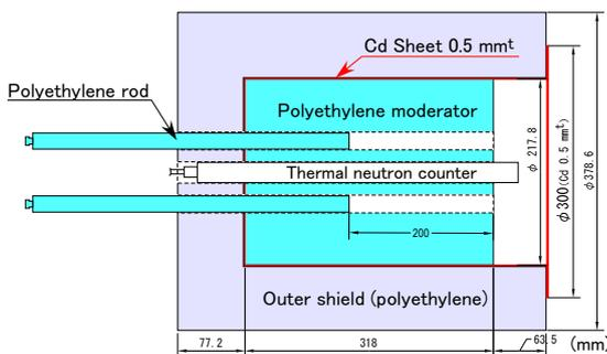
Figure 3. Schematic drawing of the Long Counter.
