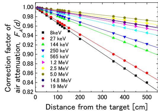
Figure 8. Correction factor of the air attenuation  $F_A(d)$  as a function of the distance from the target. These data were calculated using the MCNP-ANT code.
