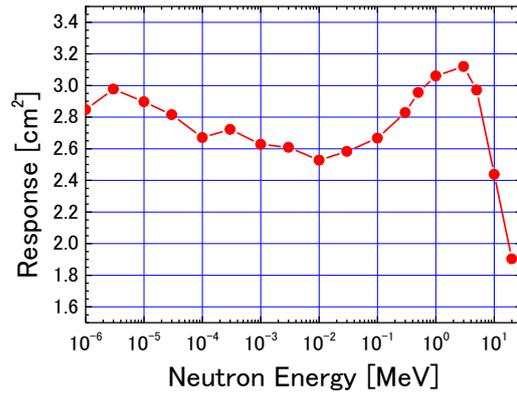
Figure 4. Response of the Long Counter calculated using the MCNP-4C code. The response was determined from the number of <sup>10</sup>B(n,α)<sup>7</sup>Li reaction in the sensitive area of the BF<sub>3</sub> counter. The shape of the response curve for the <sup>3</sup>He counter is quite similar to that of the BF<sub>3</sub> counter.
