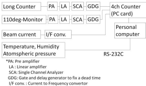
Figure 7. Block diagram of the developed neutron fluence monitoring system.
