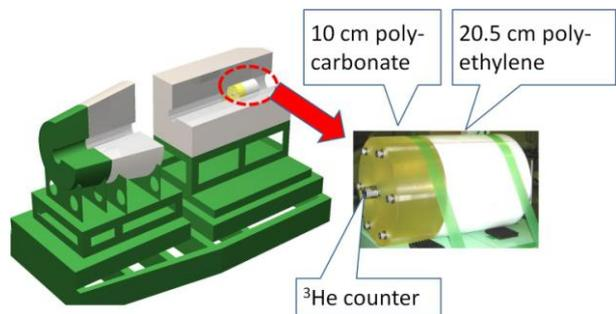
Figure 5. Schematic drawing and photograph of the 110deg-monitor installed in the collimator for time-of-flight measurement.
