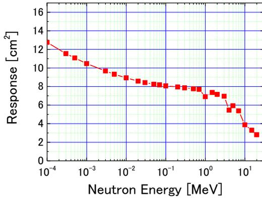
Figure 6. Response of the 110deg-monitor calculated by using the MCNP-4C code. The response was determined from the number of  ${}^3\text{He}(n,p){}^3\text{H}$  reaction in the sensitive area of the  ${}^3\text{He}$  counter.
