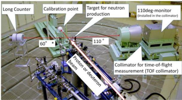
Figure 2. Photograph in the mono-energetic neutron fields. \*In the 14.8 and 19 MeV fields, the Long Counter is placed at 90 degree angle to the beam line.
