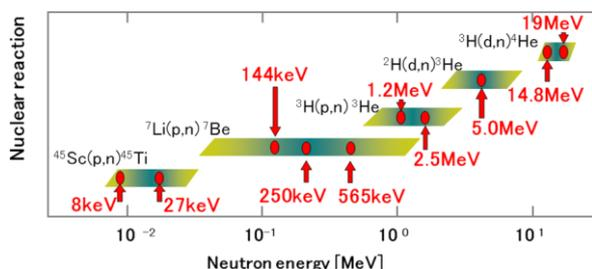
Figure 1. Available energy points and nuclear reactions employed for neutron production in the mono-energetic neutron calibration fields.
