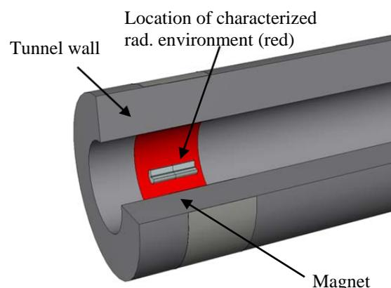
Figure 2. Illustration of the simplified accelerator tunnel geometry implemented in FLUKA in order to characterize the radiation environment at different locations. The red surface depicts the volume close to the tunnel wall that was studied as an exemplary radiation environment (ID 4 from Table 1).
