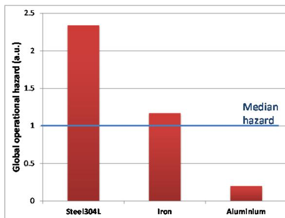
Figure 3. Comparison of the global operational hazard, based on residual dose rates, of steel 304L (0.1 wt% of Cobalt), pure iron and aluminium located next to a magnet in the LHC. 20 years of irradiation have been assumed.
