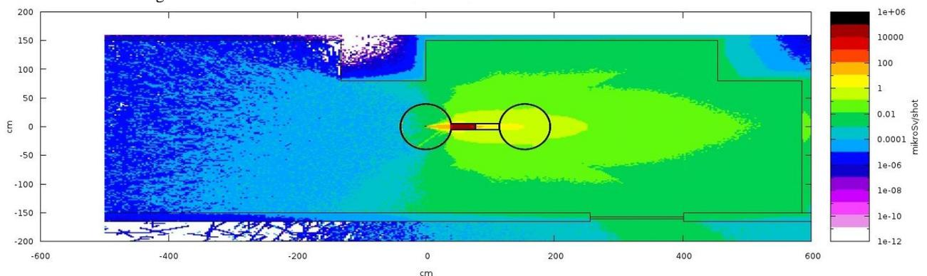
Figure 3. Distribution of calculated dose equivalent (µSv) per one shot of 100 MeV electron beam of 6.24.10<sup>6</sup> primaries, on the beam level only.
