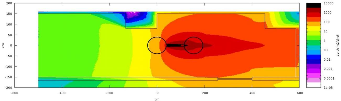
Figure 2. Calculated total photon fluence (particle/cm<sup>2</sup>) per one shot of 100 MeV electron beam of 6.24.10<sup>6</sup> primaries, averaged across the full hall height.
