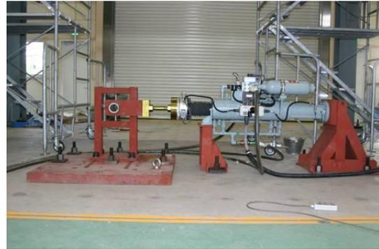
**Fig. 7** Hybrid experiment for a piping support
