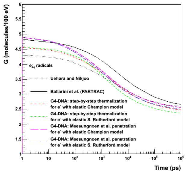
**Fig. 2** Prototype results on  $\text{e}_{\text{aq}}^-$  radiochemical yields (molecules/100 eV) from 1 MeV incident electrons with respect to time (in picosecond). References: Ballarini *et al.* (PARTRAC),<sup>3</sup>) S. Uehara and H. Nikjoo.<sup>6</sup>)
