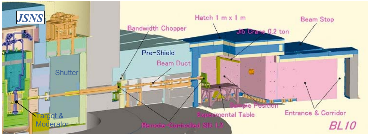
Fig. 1 Three dimensional cross sectional view of NOBORU
