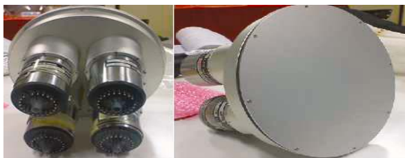
Fig. 8 The housing of large area composite stilbene scintillator
