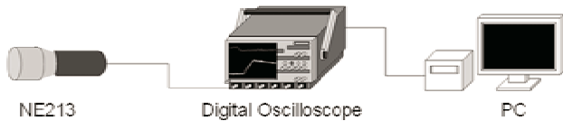
Fig.2 Schematic view of data acquisition system consisting of NE213 neutron detector, digital oscilloscope Wavepro 7000, and personal computer (PC).
