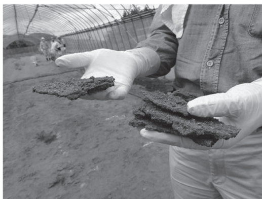
Figure 2 Slices of soil scraped off at farmland for greenhouses after being solidified using polyion complexes for decontamination 1)
