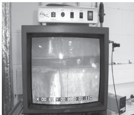
Fig. 1 Magnified image of fibres on beam line as viewed using a microscope and monitor display.
