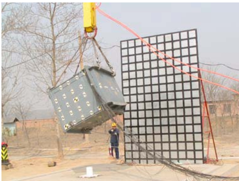
Fig.6 The container subjected to the free drop test II
